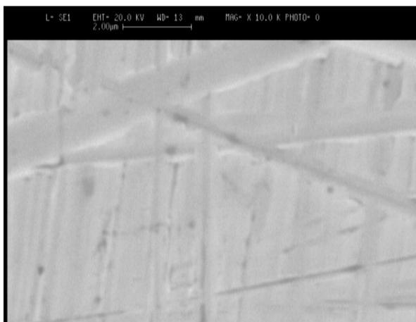
**Figure 11:** Microstructures (SEM) of species coated with multilayers of PDADMA/PSS and 1mM Benzotriazole on treated mild steel.
