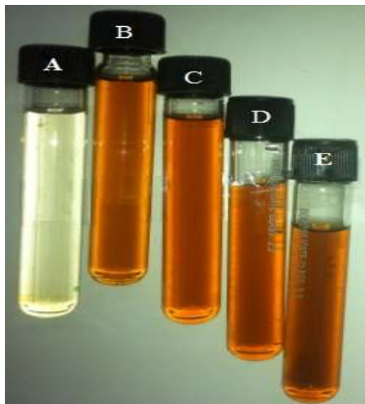
Figure 1. The color change of the mustard exudates upon the formation of AgNPs from different concentrations of A: 0, B: 1, C: 2.5, D: 4, and E: 5 mM AgNO 3 .
